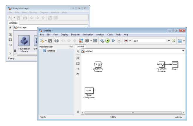
By default, the model name is not specified, the model contains a Solver Configuration block with the default solver set to ode15s, a Simulink-PS
